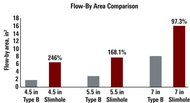
*The flow-by area of the Don-Nan slimhole tubing anchor is significantly increased when compared with the Type B tubing anchor, resulting in enhanced rod lift system efficiency.*
